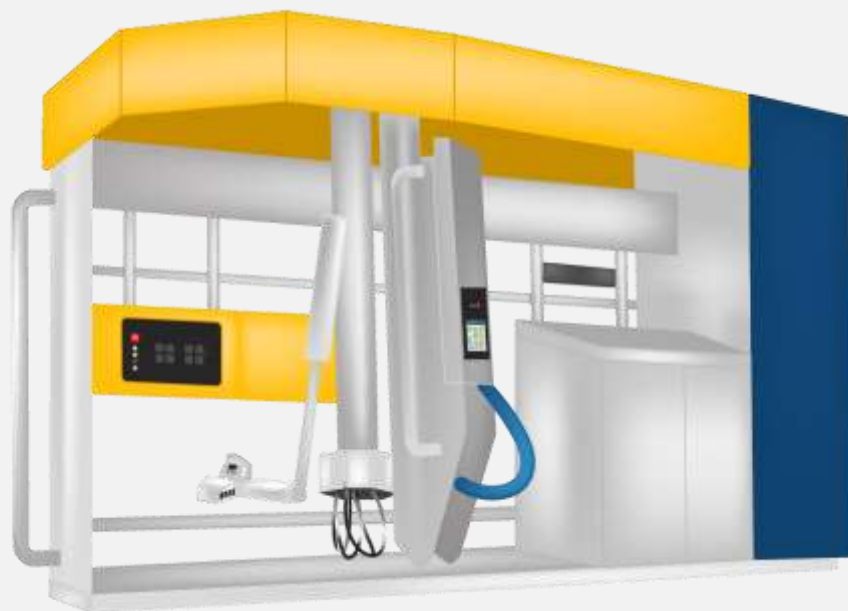
Figure 2. A Model of an Automated Milking System
